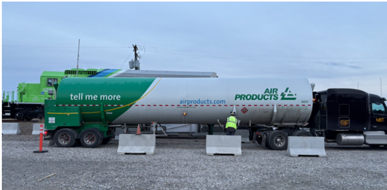
Figure 25 - L to G Refueler on-site in Lethbridge, AB.
