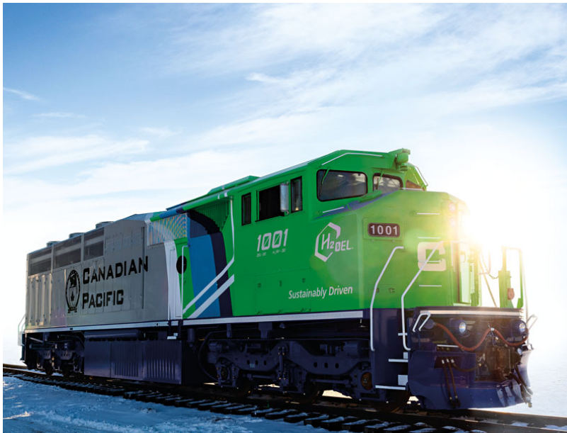
Figure 8 - CP 1001 hydrogen fuel cell battery hybrid locomotive. North America's first for line-haul operation.
