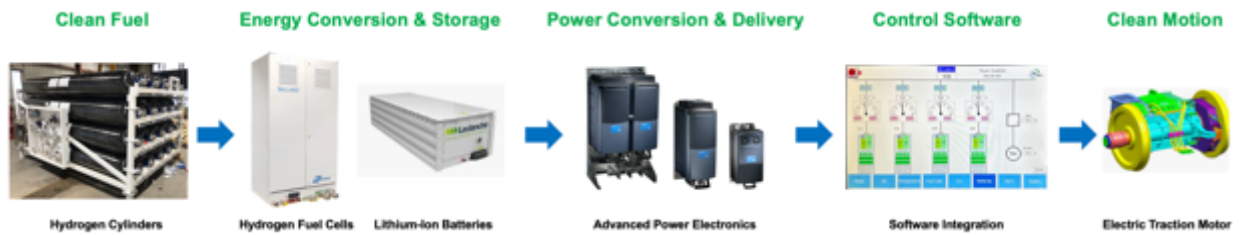
Figure 6 - High-level summary of the process of using hydrogen gas to drive a locomotive electric traction motor and the overall locomotive architecture.
