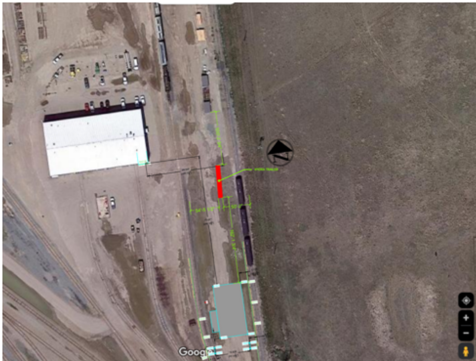
Figure 19 - Fixed-point refueling infrastructure site plan.
