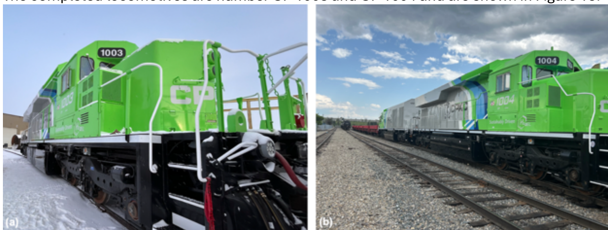
Figure 15 – Completed CP 1003 (a) and CP 1004 (b) hydrogen fuel cell battery locomotives.
