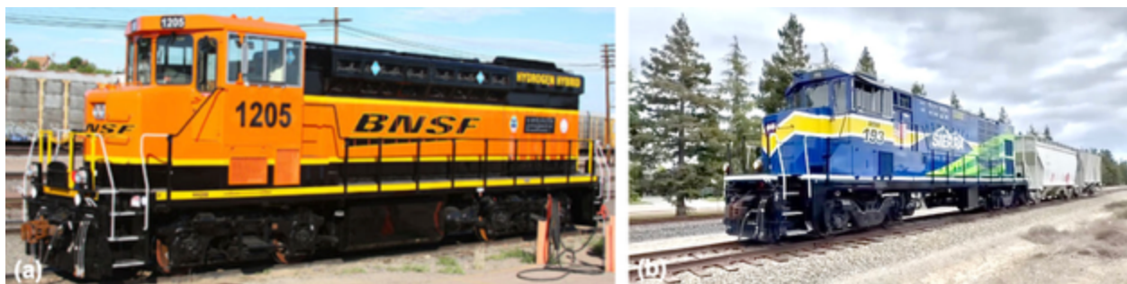
Figure 7 – (a) BNSF and (b) Sierra Northern Hydrogen Hybrid switcher locomotive (RailPicture.net photo Nathan Zachman, Trains)
