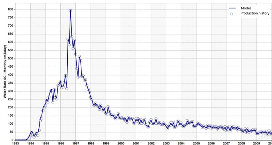
Figure 5: Comparison between production water rate at the field level from historical production data and the history-matched model, demonstrating the accuracy of the history matching process.
