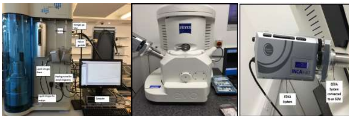
Figure 8: The Quantachrome Model 2013 Automated Gas Sorption Analyzer (Left); the Zeiss EVO Scanning Electron Microscope used for the SEM Imaging (Middle) and Energy Dispersive X-ray Analysis System (Oxford Instruments INCAx-act) used for the EDAX Analysis (Right)
