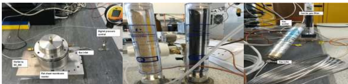
Figure 9: Condenser and Gas-Liquid Separator (Left); Perkin Elmer Moisture Trap from Llantrisant, UK (Middle) and Chemical Ionization Gas Purifier (Right)
