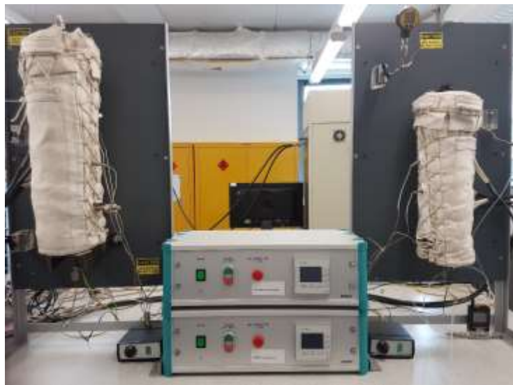
Figure 6: Photograph of the Two Membrane Reactors Enclosed in the Heating Furnace (Heating Jacket) with Power Controllers between the Reactors and Showing the Thermocouples
