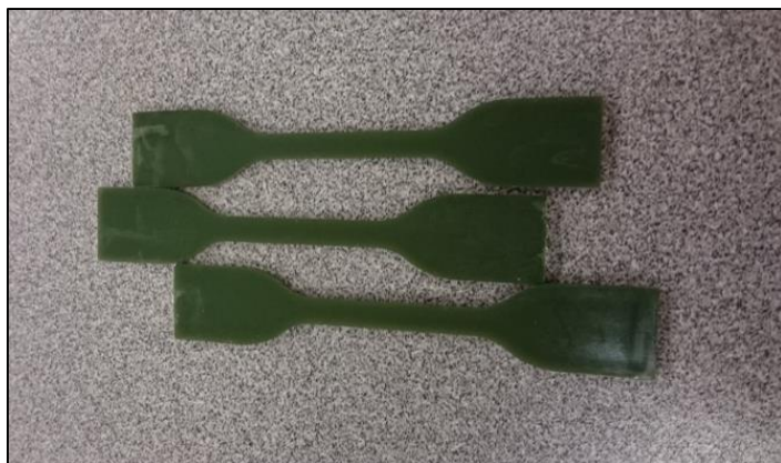
Figure 14. Photograph of HDPE samples with 0.03% wt. dosage of carbon nanoplatelets with a 0.3% dosage of colourant.
