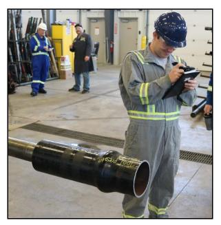
This is the same piece of test casing a few minutes later. Here the 7" casing has been expanded to over 8.5" OD. Before the CET is deployed in a wellbore, Winterhawk secures a piece of casing of the same size, thickness and grade as that in the well to determine whether or not the tool has the power to expand against cement and the anticipated performance in a that casing in the wellbore.
