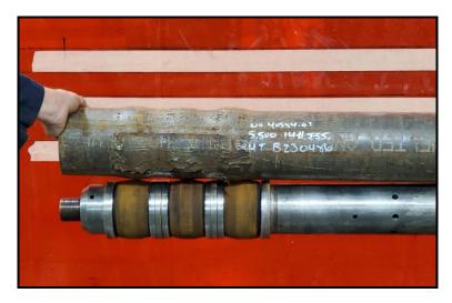
Winterhawk's project engineer wanted more surface area of expanded casing for enhanced cement compression.
