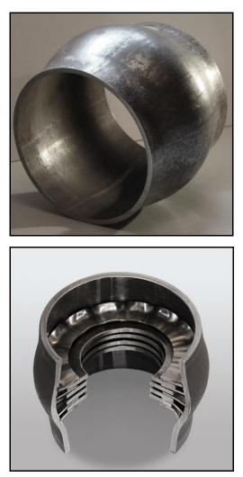
However, setting this assembly in the wellbore then releasing from its proved difficult. It was finally concluded after significant field trials that a preferable assembly would be retractable, then retrievable. In 2018 the pleated steel ring was replaced with an expandable elastomer element.
