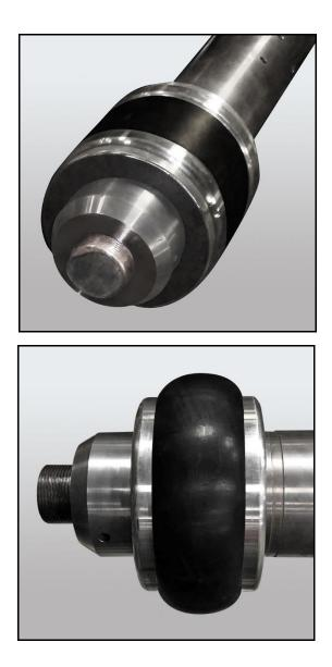
The first test well using this assembly was conducted near Lloydminster in a test well for a major operator in the summer of 2018. However, post-test multi-finger casing caliper logs revealed that the tool did not have sufficient power to expand the wellbore casing against cement at 100 tons of force. The operator had committed to funding a five-well testing and development program.
