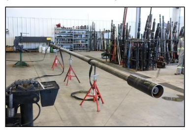
The 4.20" OD tool for 7" (177.8 mm) casing converts 4,000 psi of hydraulic pressure into an outward force of 440,000#. This illustration is the setting tool with a piece of test casing ready for expansion.
