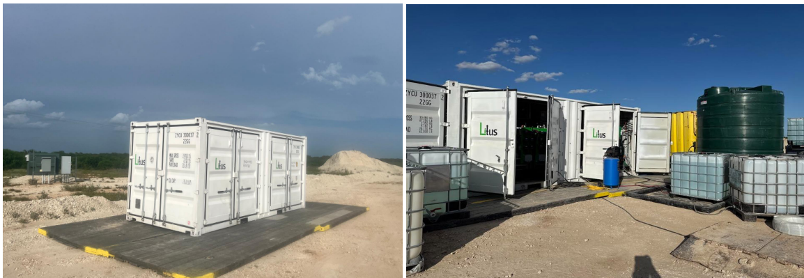
Figure 2: Litus LiNC Pilot Unit Installed in the Field with Feed Tanks
