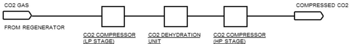
**FIGURE 4.5 CO<sub>2</sub> COMPRESSOR**
