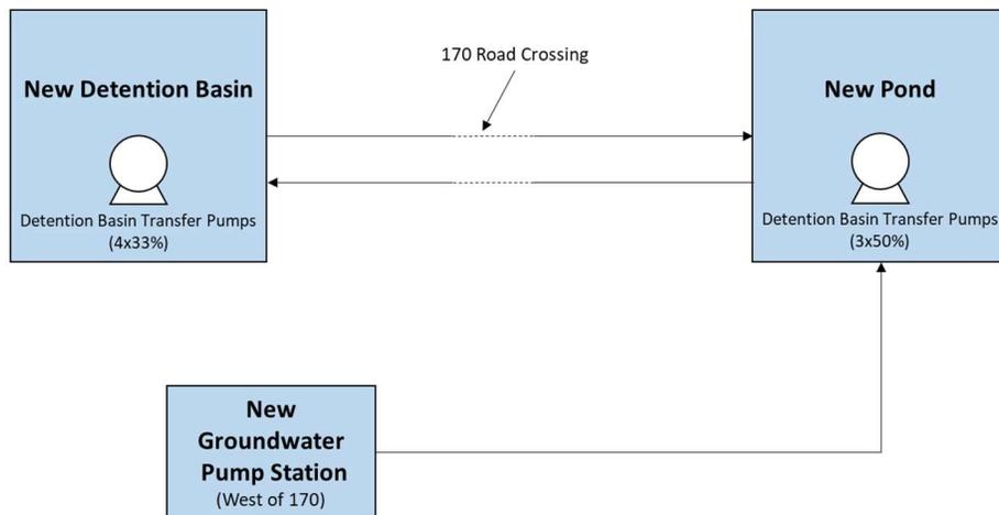
**FIGURE 8.5 POND TRANSFER DIAGRAM**
