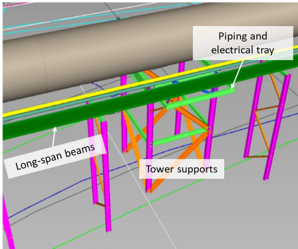
**FIGURE 3.4 TYPICAL DUCT, PIPING, AND TRAY SUPPORTS**
