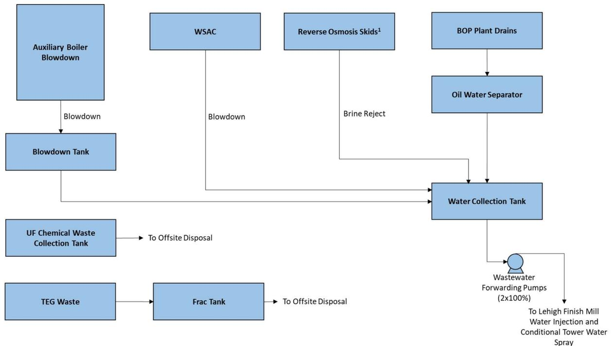
**FIGURE 8.4 WASTEWATER PROCESS FLOW DIAGRAM**
