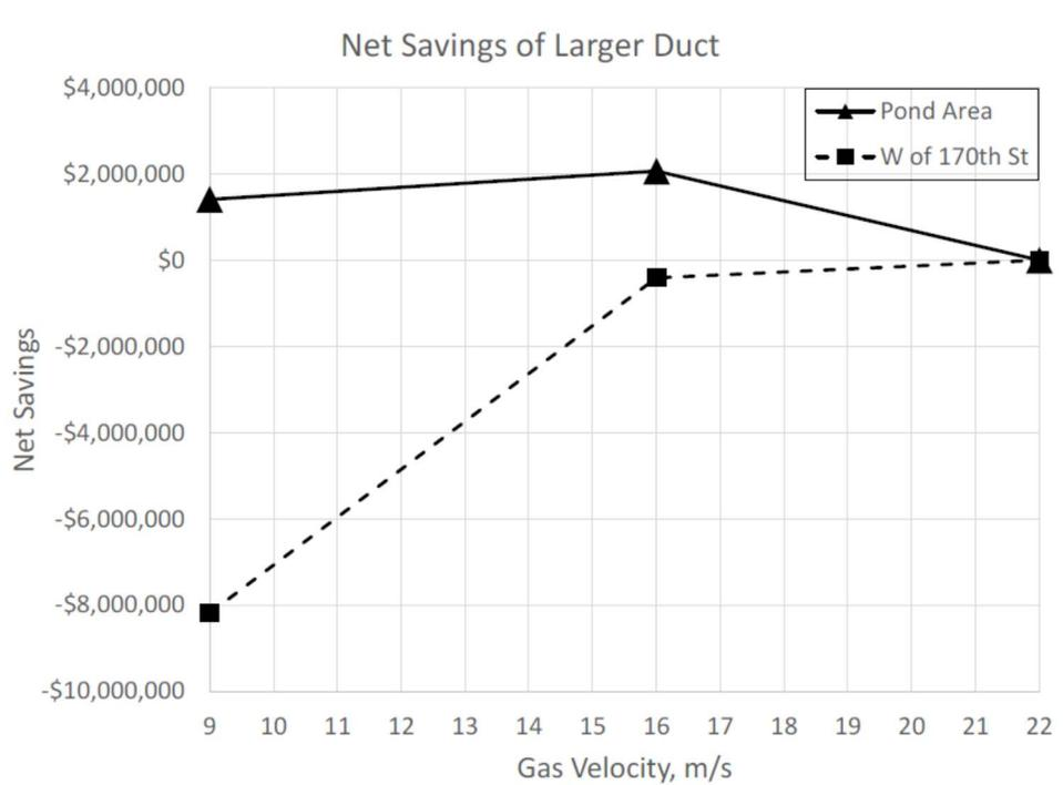
FIGURE 3.3 NET SAVINGS FOR LARGER DUCT DIAMETERS
