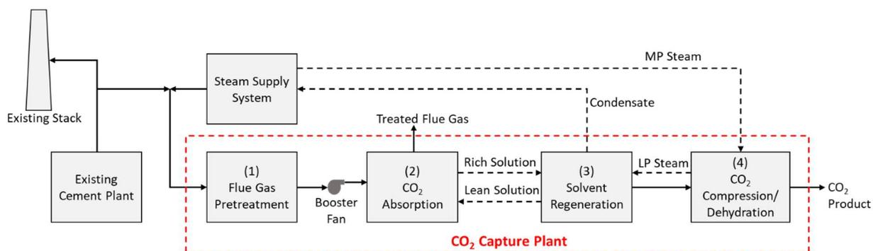
FIGURE 4.1 BLOCK FLOW DIAGRAM OF THE CO<sub>2</sub> CAPTURE PLANT
