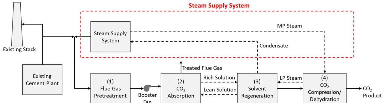
**FIGURE 7.1 SIMPLIFIED DIAGRAM OF CO<sub>2</sub> CAPTURE AND COMPRESSION PROCESS WITH STEAM SUPPLY SYSTEM HIGHLIGHTED**
