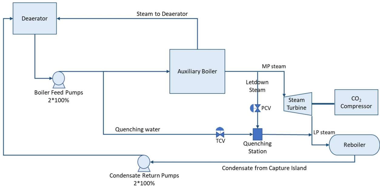
**FIGURE 7.2 PROCESS FLOW DIAGRAM FOR STEAM SUPPLY SYSTEM**
