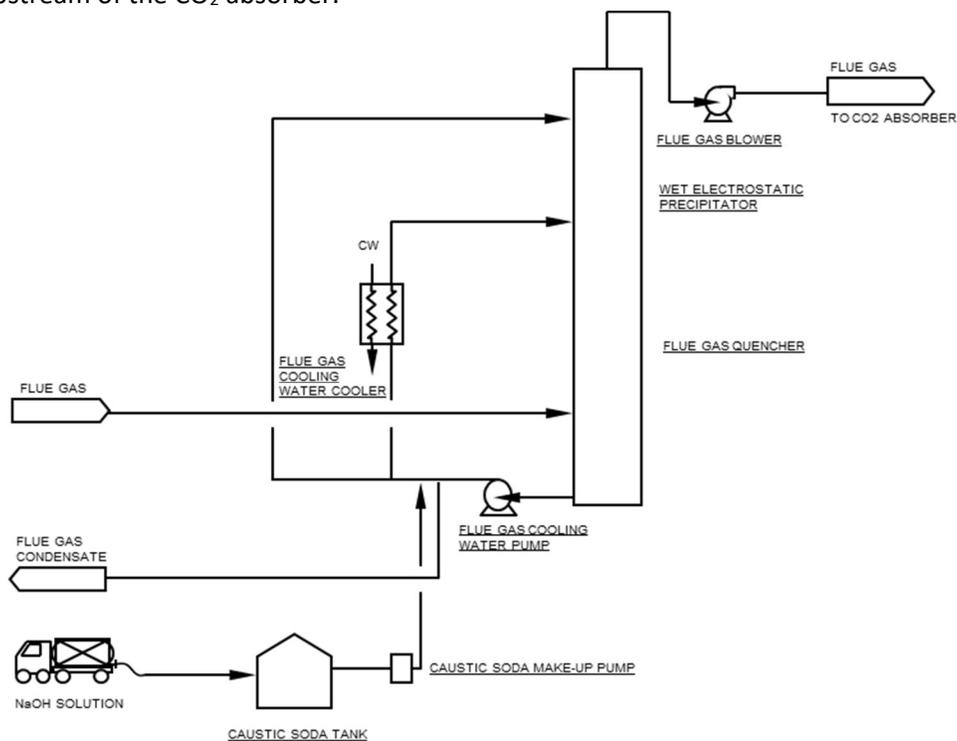
FIGURE 4.2 FLOW DIAGRAM FOR FLUE GAS PRETREATMENT
