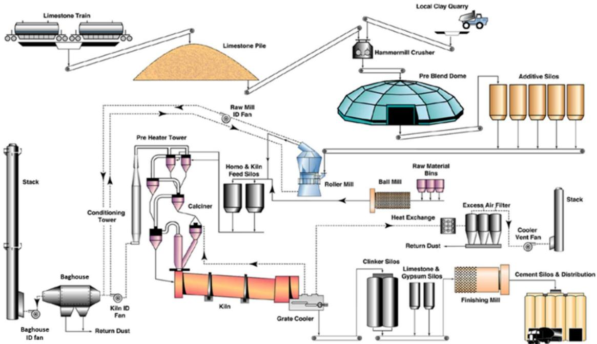
**FIGURE 1.3 PROCESS FLOW DIAGRAM OF CEMENT PRODUCTION AT LEHIGH**
