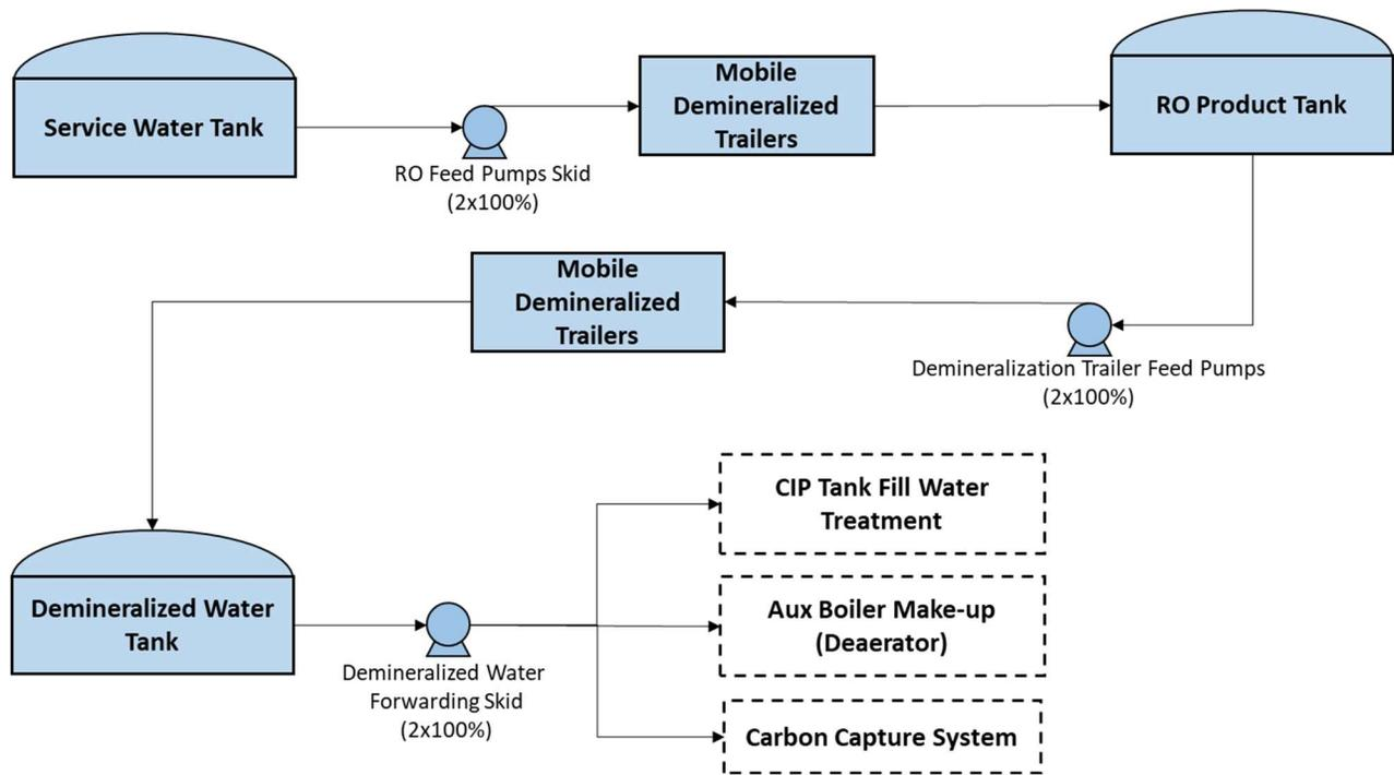
**FIGURE 8.1 DEMINERALIZED WATER FLOW DIAGRAM**
