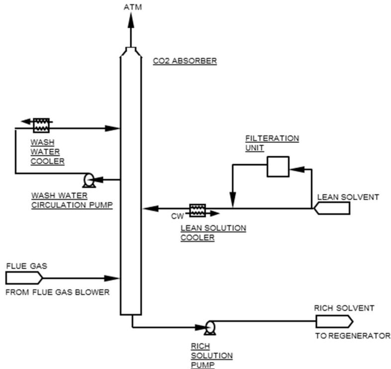
FIGURE 4.3 CO<sub>2</sub> ABSORBER
