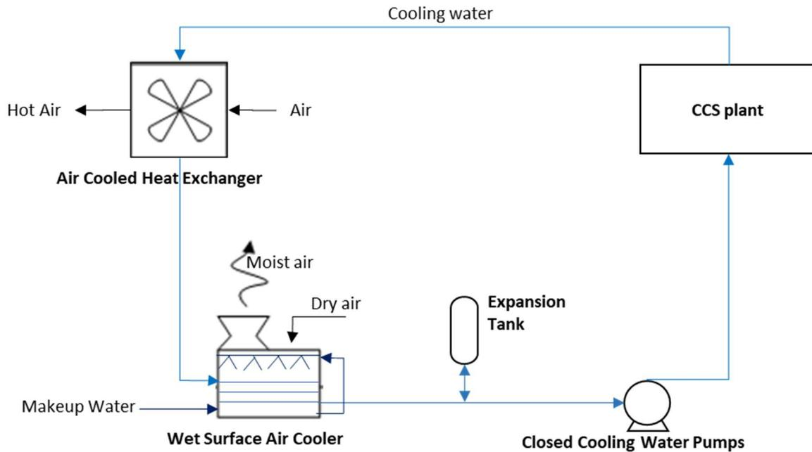
FIGURE 5.2 SIMPLIFIED FLOW DIAGRAM OF SINGLE LOOP HYBRID COOLING SYSTEM
