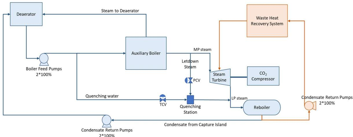
**FIGURE 7.3 SIMPLIFIED DIAGRAM OF STEAM SUPPLY SYSTEM**
