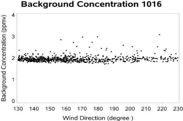
Figure 2: Variability in the background methane concentration as a function of wind direction. At the edges of the wind direction there was no undesirable spikes, which indicates no contamination of the concentration from adjacent pens of animals. The number 1016 indicates the laser number.
