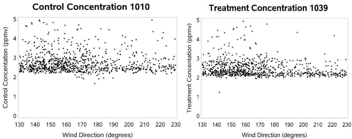
Figure 3: Methane concentrations downwind of the Control (left graph) and Treatment (right graph) pen block showing greater concentrations above background due to enhancement from the cattle. The numbers 1010 and 1039 indicate the laser number.
