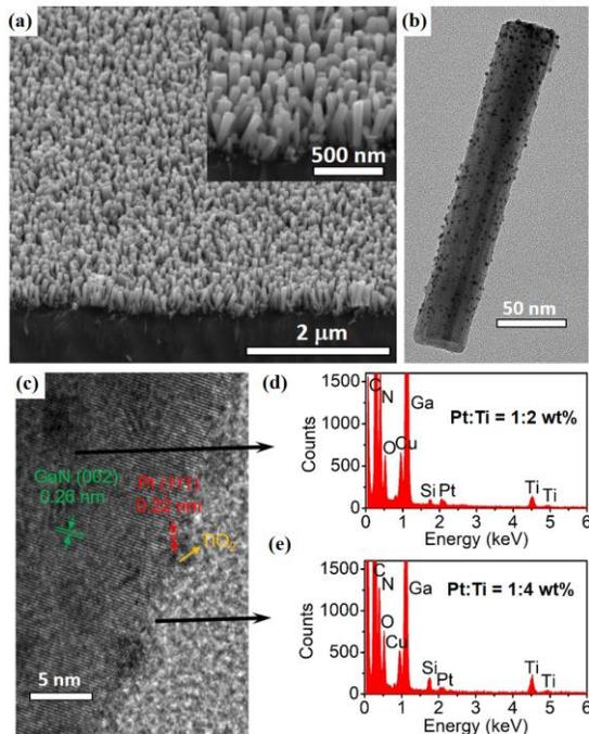
**Figure 6.** Characterization of Pt-TiO<sub>2</sub>/GaN/n<sup>+</sup>-p Si sample. (a) 45°-tilted SEM image shows GaN nanowire growth vertically on the Si substrate, (b) TEM image illustrates Pt nanoparticles distributed uniformly on the GaN nanowire surface, (c) HRTEM image, and EDX analysis of the
