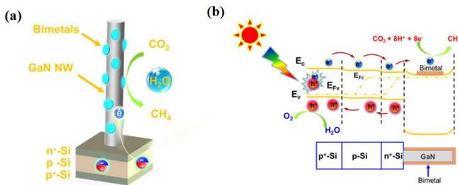
**Figure 3.** (a) Schematic illustration and (b) energy diagram of bimetallic co-catalysts supported on GaN nanowires/Si for photoelectrochemical CO<sub>2</sub> reduction towards CH<sub>4</sub>.
