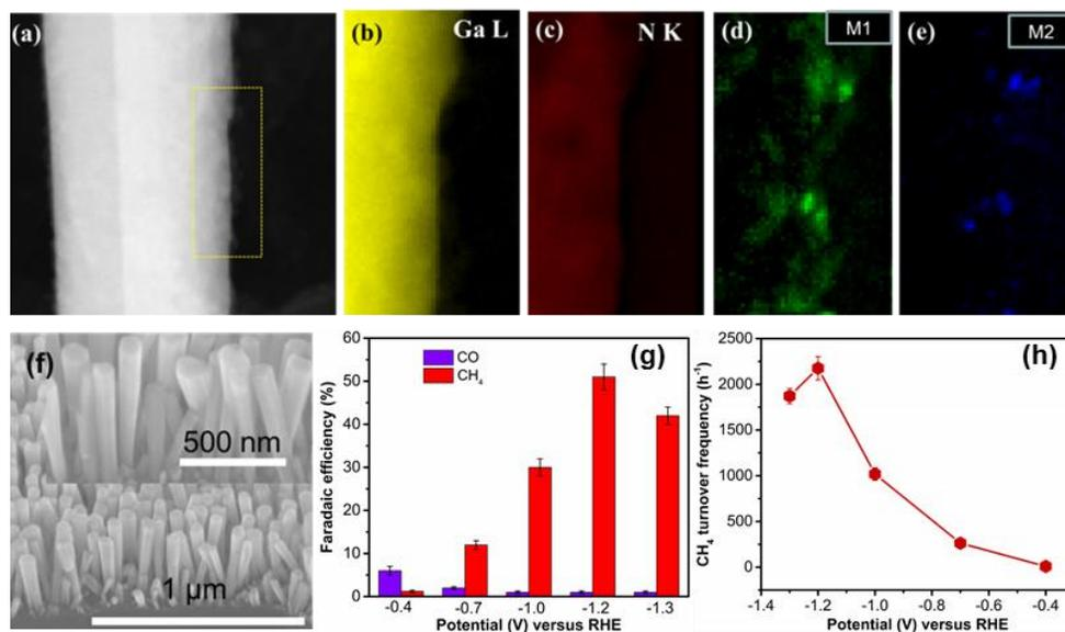
**Figure 4.** Structure of photoelectrode and photoelectrochemical performance for CO<sub>2</sub> conversion to methane. (a) HAADF-STEM image of GaN nanowire modified with bimetallic co-catalysts. The elemental distribution mapping of (b) Ga, (c) N, (d) M1 and (e) M2. (f) SEM images of GaN nanowire modified with bimetallic co-catalysts. Dependence of (g) Faradaic efficiency, and (h) turnover frequency number of methane on applied potentials.
