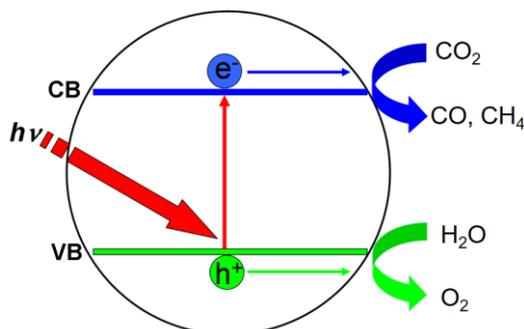
**Figure 1.** Schematic illustration of the mechanism for the photo-reduction of  $CO_2$ .
