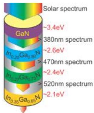
**Figure 2.** Schematic illustration of multi-band InGaN to split solar spectrum.
