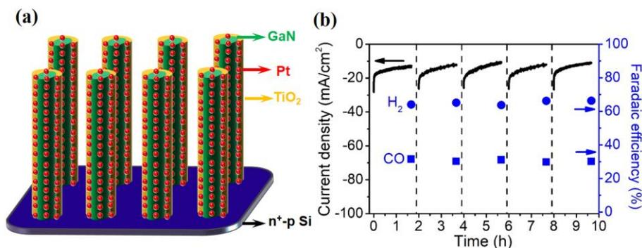
**Figure 5.** (a) Schematic illustration and (b) performance of Pt-TiO<sub>2</sub>/GaN/n<sup>+</sup>-p Si photoelectrode.
