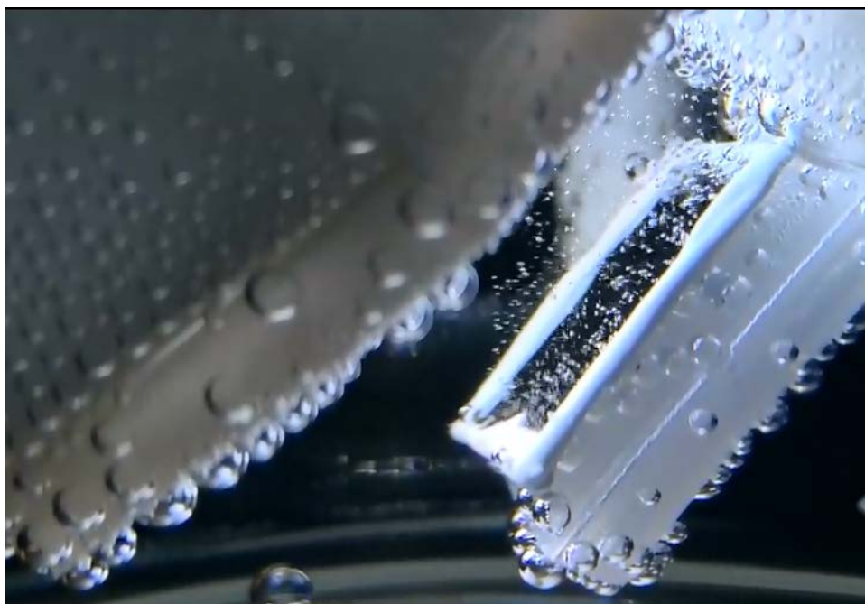
Figure 3.4.3: Large surface area prototype demonstrating spontaneous water splitting.
