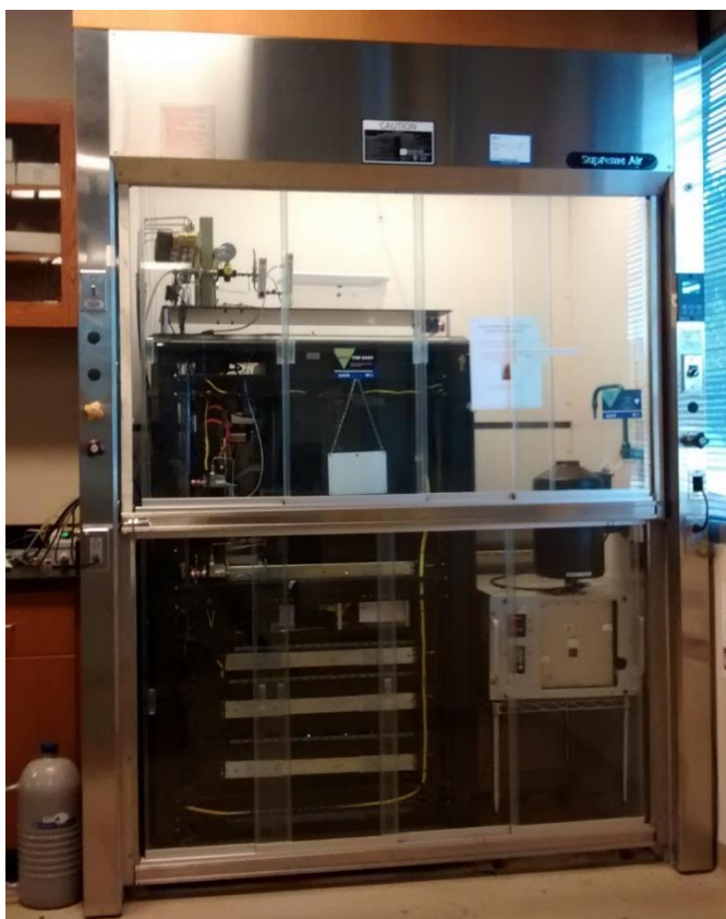
Figure 10. The microreactor packed-bed system in a walk-in hood.
