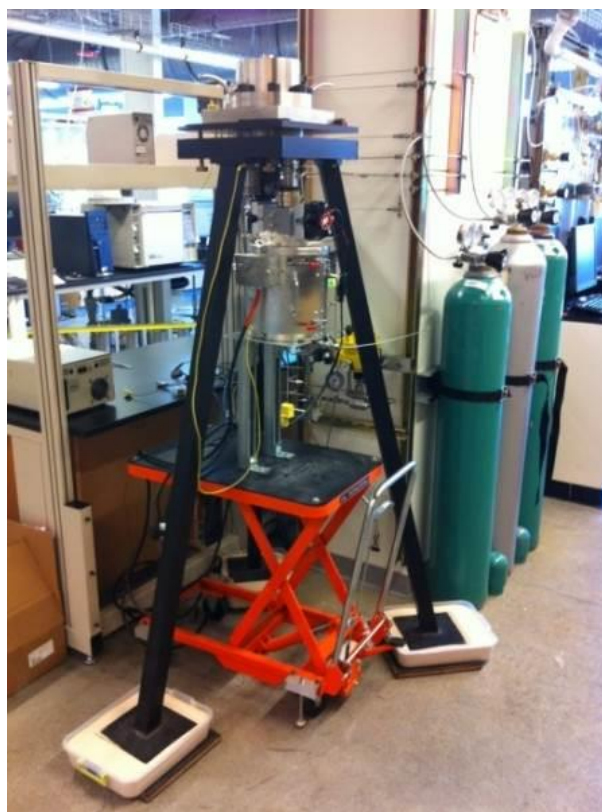
Figure 9. HP-TGA for catalyst performance testing.
