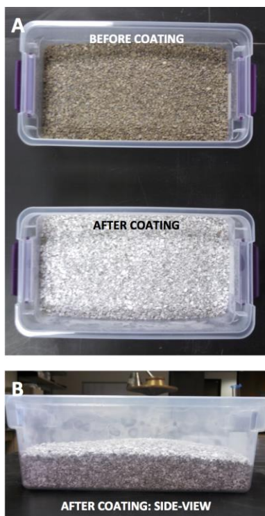
Fig. 9 Examples of fine, lightweight \text{CaCO}_3 -coated aggregate produced in Blue Planet's pilot plant. (A) Shows the difference in aggregate before and after coating. (B) A side-view of the coated aggregate in (A).
