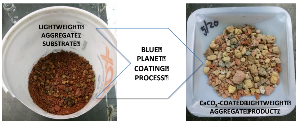
Fig. 11 Images of what the CarbonMix CaCO 3 -coated aggregate might look like inside its bag (Figure 12) on the shelves at home improvement stores anywhere in the world. This particular product was made in a pilot reactor and is ASTM C330 specifiable aggregate.
