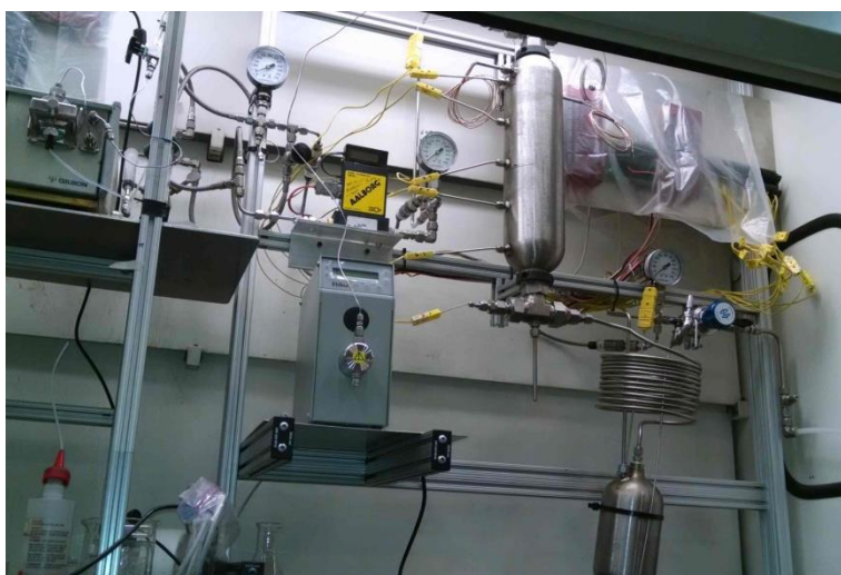
Final Phase B hydrogenation reactor system.
