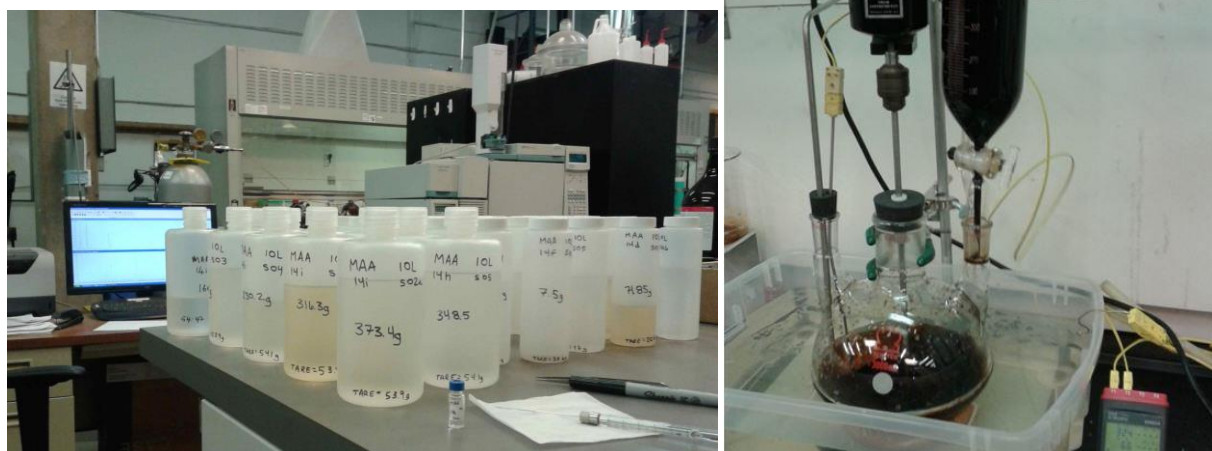
Product samples from hydrogenation experiments (left) and MAA synthesis from diketene (right).
