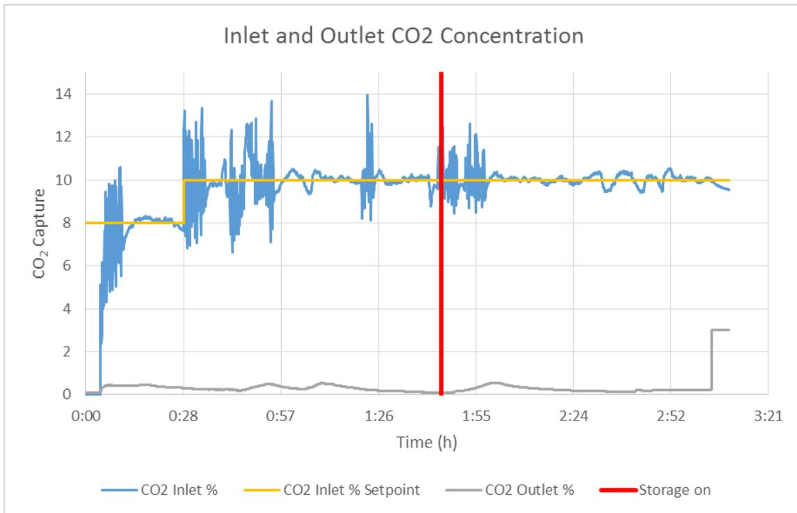
Figure 21. CO<sub>2</sub> inlet and outlet percentages during CCC ES<sup>TM</sup> testing. For the first portion of the test (left of the red line), we stored energy. The second part of the test (right of the red line), we captured CO<sub>2</sub> only using the stored LNG.
