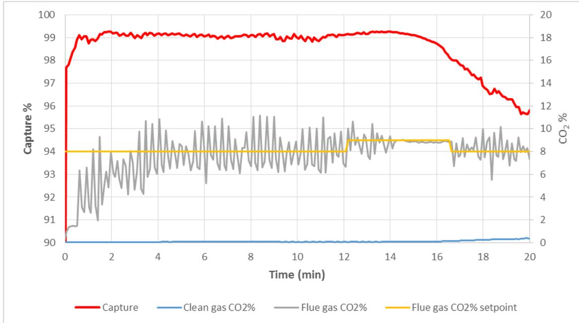
Figure 23. 99% CO<sub>2</sub> capture demonstrated for 15 minutes. CO<sub>2</sub> inlet and outlet percentages are also shown (right axis).
