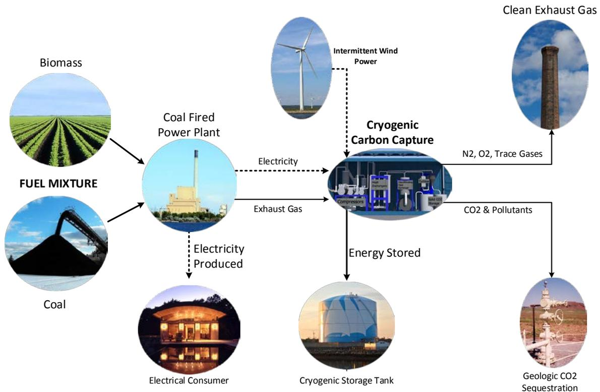
Figure 28. CCC ES™ integration into the grid resulting in a negative carbon footprint for electrical power production.
