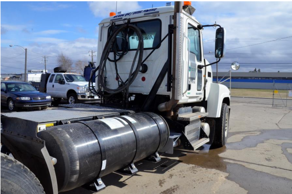
Figure 6: Edmonton refuse hauler heavy duty truck with Hitec dual fuel system
