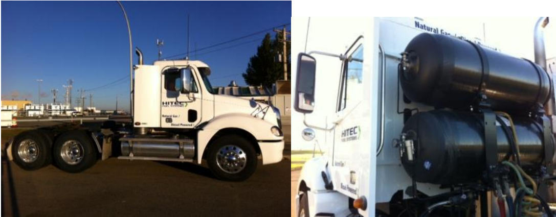
Figure 3: Hitec dual fuel Freightliner demonstration truck
