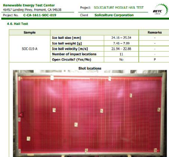
Figure 12: Results of hail test of 1m x 2m Soliculture module. Module passed impact of 11 25mm ice balls traveling at 22m/s
