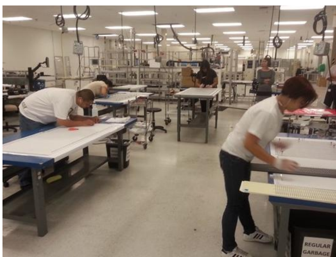
Figure 5: Manufacturing 300 Soliculture panels at Solaria in Fremont, CA in June of 2015. Workers lay out the encapsulant and strings before lamination.
