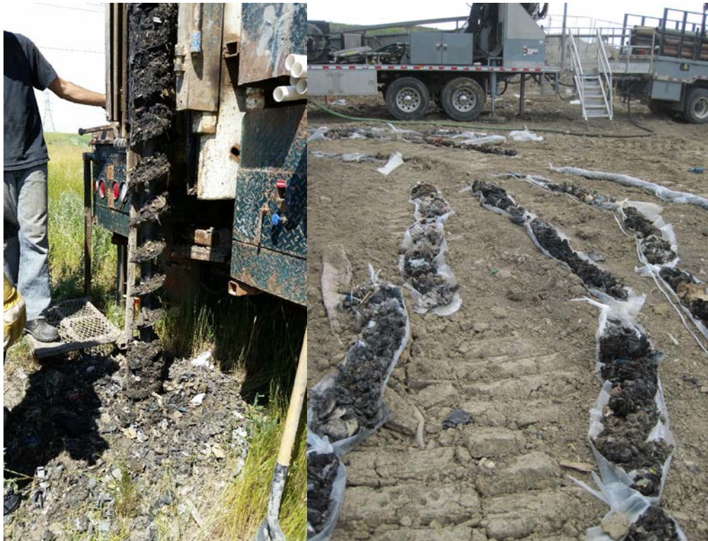
Figure 3. Auger drilling operation (left) and resultant MSW sample (right) - courtesy of the City of Lethbridge.
