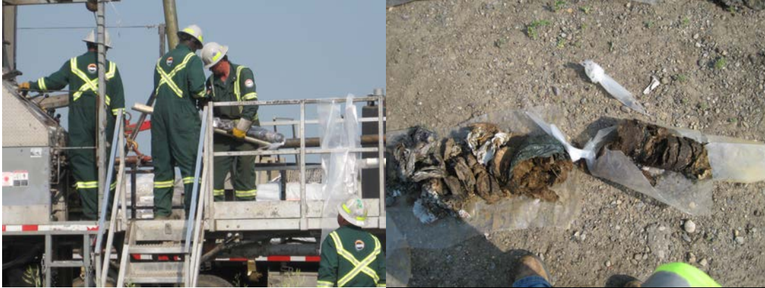
Figure 4. Core drilling operation (left) and MSW core drilled sample (right) - courtesy of the City of Lethbridge.
