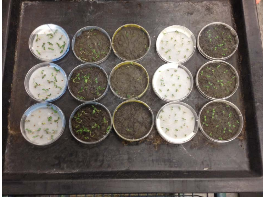
Photograph 4: Germination experiment with filter paper (controls) and Alberta soils.
