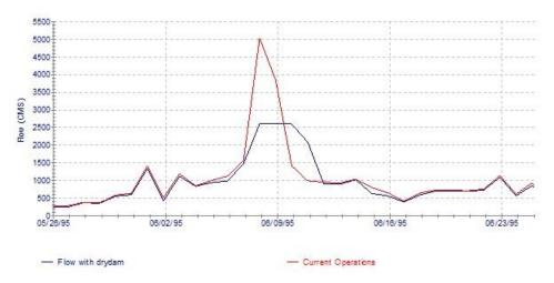
Figure 51: Flow to Oldman Mouth with dry dam in place (1995)
