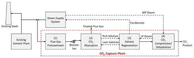
FIGURE 4.1 BLOCK FLOW DIAGRAM OF THE CO2 CAPTURE PLANT
