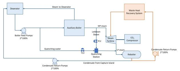
FIGURE 7.3 SIMPLIFIED DIAGRAM OF STEAM SUPPLY SYSTEM
