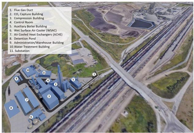
FIGURE 9.2 WEST OF 170 LOCATION CCS AND BOP FACILITIES LAYOUT
