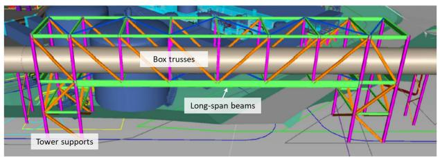
FIGURE 3.5 TYPICAL TRUSSED ROAD CROSSING
