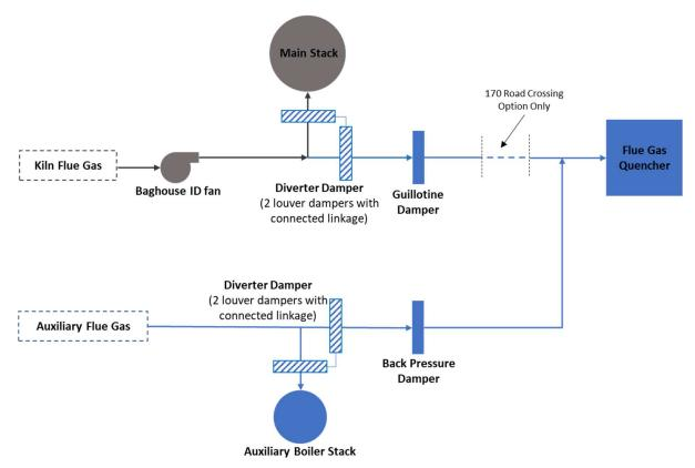
FIGURE 3.2 FLOW DIAGRAM OF FLUE GAS SUPPLY SYSTEM
