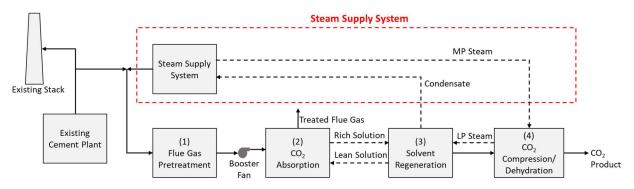
FIGURE 7.1 SIMPLIFIED DIAGRAM OF CO<sub>2</sub> CAPTURE AND COMPRESSION PROCESS WITH STEAM SUPPLY SYSTEM HIGHLIGHTED
