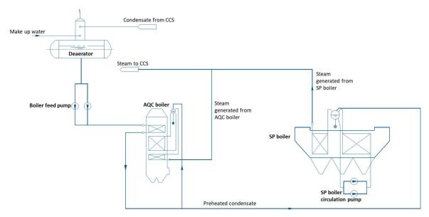
FIGURE 7.5 FLOW DIAGRAM OF WASTE HEAT RECOVERY SYSTEM (WASTE AND STEAM)
