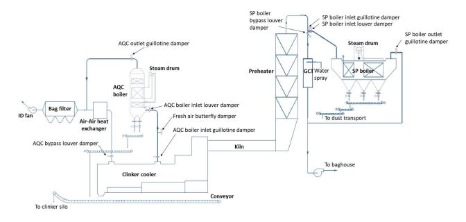
FIGURE 7.4 FLOW DIAGRAM OF WASTE HEAT RECOVERY SYSTEM (GAS)
