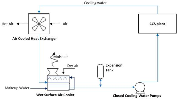
FIGURE 5.2 SIMPLIFIED FLOW DIAGRAM OF SINGLE LOOP HYBRID COOLING SYSTEM
