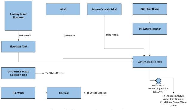
FIGURE 8.4 WASTEWATER PROCESS FLOW DIAGRAM
