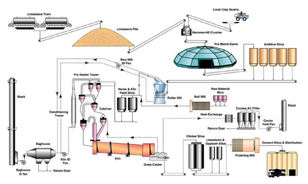
FIGURE 1.3PROCESS FLOW DIAGRAM OF CEMENT PRODUCTION AT LEHIGH
