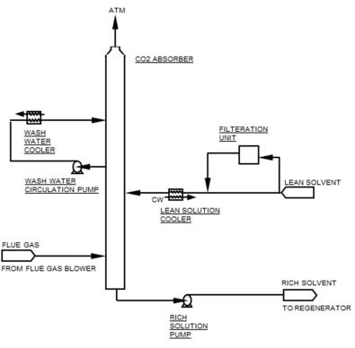
FIGURE 4.3 CO<sub>2</sub> ABSORBER
