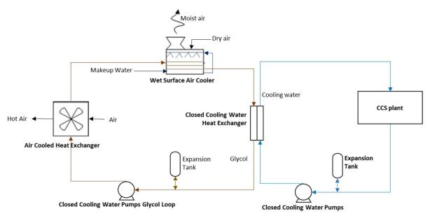
FIGURE 5.3 SIMPLIFIED FLOW DIAGRAM OF DUAL LOOP HYBRID COOLING SYSTEM
