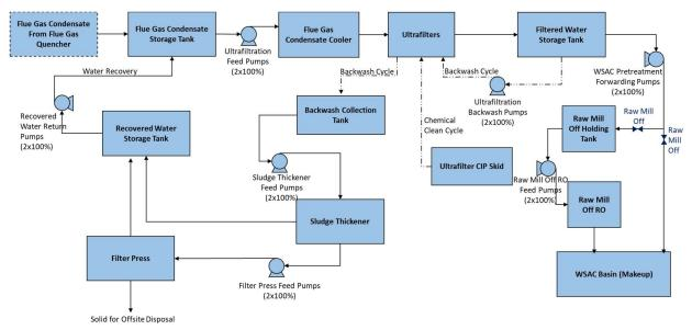
FIGURE 8.3 PROCESS FLOW DIAGRAM FOR WATER TREATMENT PLANT
