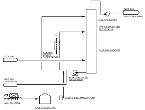
FIGURE 4.2 FLOW DIAGRAM FOR FLUE GAS PRETREATMENT
