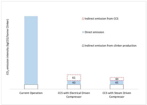
FIGURE 12.1 CO<sub>2</sub> EMISSION INTENSITY PER TONNE OF CLINKER
