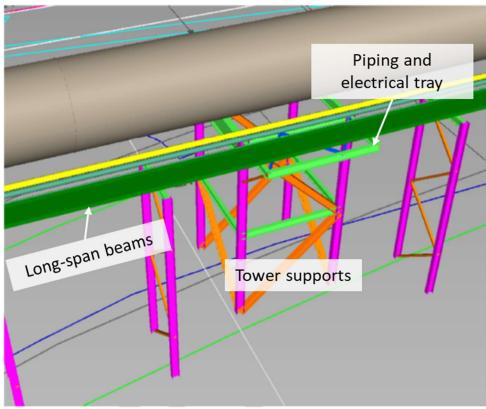
FIGURE 3.4 TYPICAL DUCT, PIPING, AND TRAY SUPPORTS
