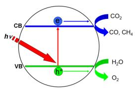
Figure 1. Schematic illustration of the mechanism for the photo-reduction of CO<sub>2</sub>.
