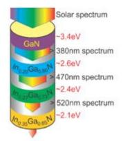
Figure 2. Schematic illustration of multi-band InGaN to split solar spectrum.
