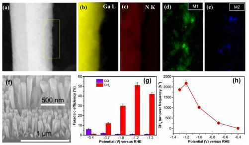
**Figure 4.** Structure of photoelectrode and photoelectrochemical performance for  $CO_2$  conversion to methane. (a) HAADF-STEM image of GaN nanowire modified with bimetallic co-catalysts. The elemental distribution mapping of (b) Ga, (c) N, (d) M1 and (e) M2. (f) SEM images of GaN nanowire modified with bimetallic co-catalysts. Dependence of (g) Faradaic efficiency, and (h) turnover frequency number of methane on applied potentials.
