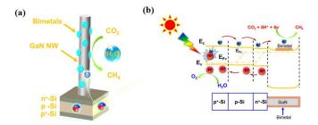
**Figure 3.** (a) Schematic illustration and (b) energy diagram of bimetallic co-catalysts supported on GaN nanowires/Si for photoelectrochemical CO<sub>2</sub> reduction towards CH<sub>4</sub>.
