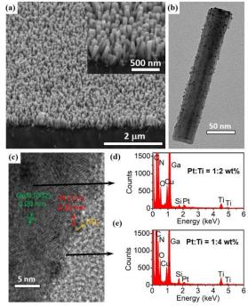
**Figure 6.** Characterization of Pt-TiO<sub>2</sub>/GaN/n<sup>+</sup>-p Si sample. (a)  $45^{\circ}$ -tilted SEM image shows GaN nanowire growth vertically on the Si substrate, (b) TEM image illustrates Pt nanoparticles distributed uniformly on the GaN nanowire surface, (c) HRTEM image, and EDX analysis of the
