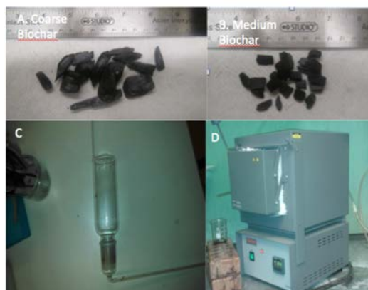
Figure 25. A. Coarse biochar, B: Medium Biochar, C: Glass Vessle, D. Muffle Furnace
