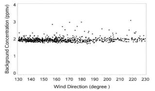
Figure 2: Variability in the background methane concentration as a function of wind direction. At the edges of the wind direction there was no undesirable spikes, which indicates no contamination of the concentration from adjacent pens of animals. The number 1016 indicates the laser number.
