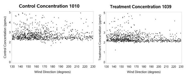
Figure 3: Methane concentrations downwind of the Control (left graph) and Treatment (right graph) pen block showing greater concentrations above background due to enhancement from the cattle. The numbers 1010 and 1039 indicate the laser number.
