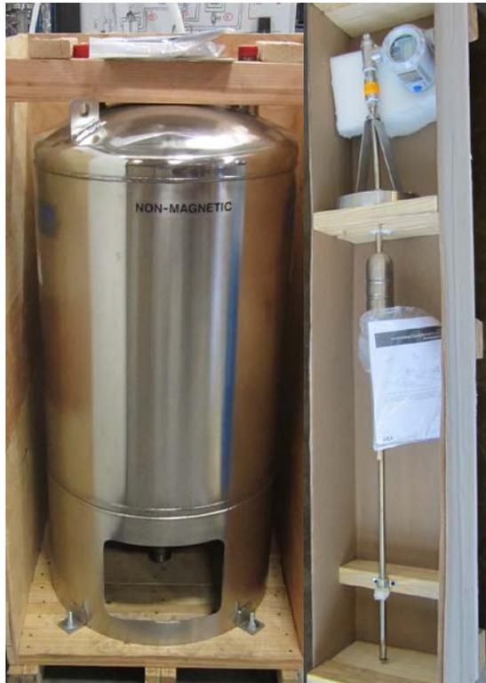
Figure 6. LNG dewar and level sensor.
