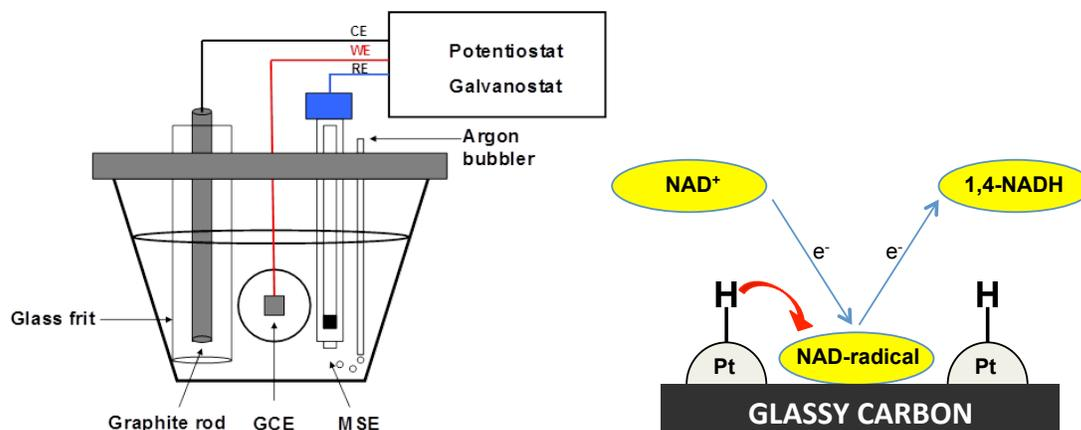
Figure 4- NADH regeneration system through electrochemical pathway
