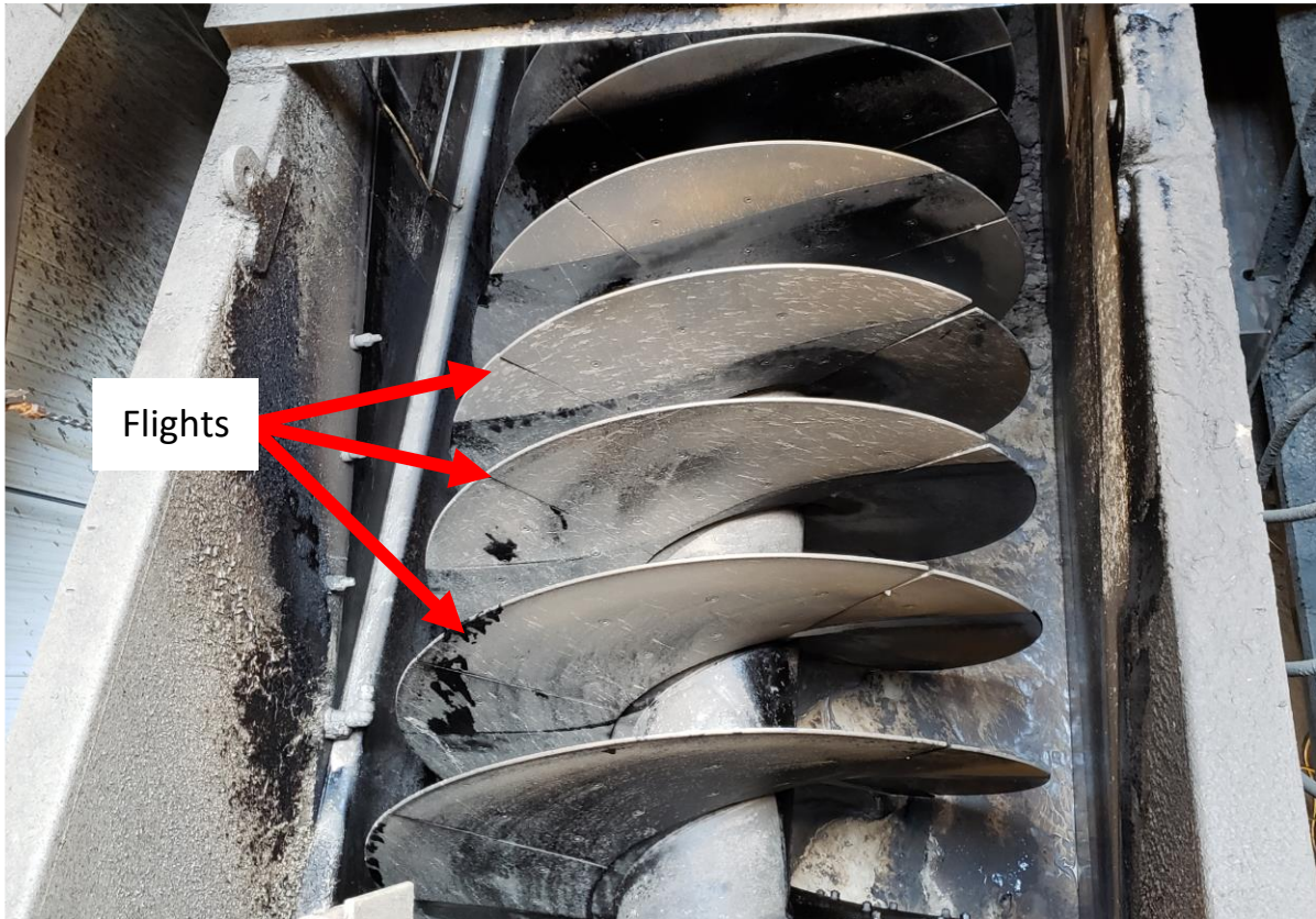
Figure D-7 Coarse screw washer flights
