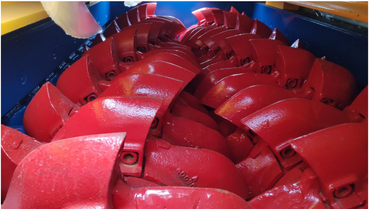
Figure D-5 Crusher teeth (Phase 3)
