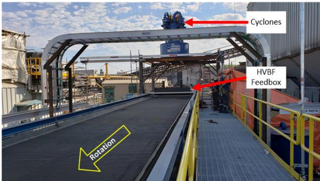
Figure D-14 HVBF installation showing location of cyclopac and HVBF feed box, filter cloth, and direction of travel. (Phase 3B during construction - note filter cloth has not been installed in lower photo and the carrying belt can be seen)
