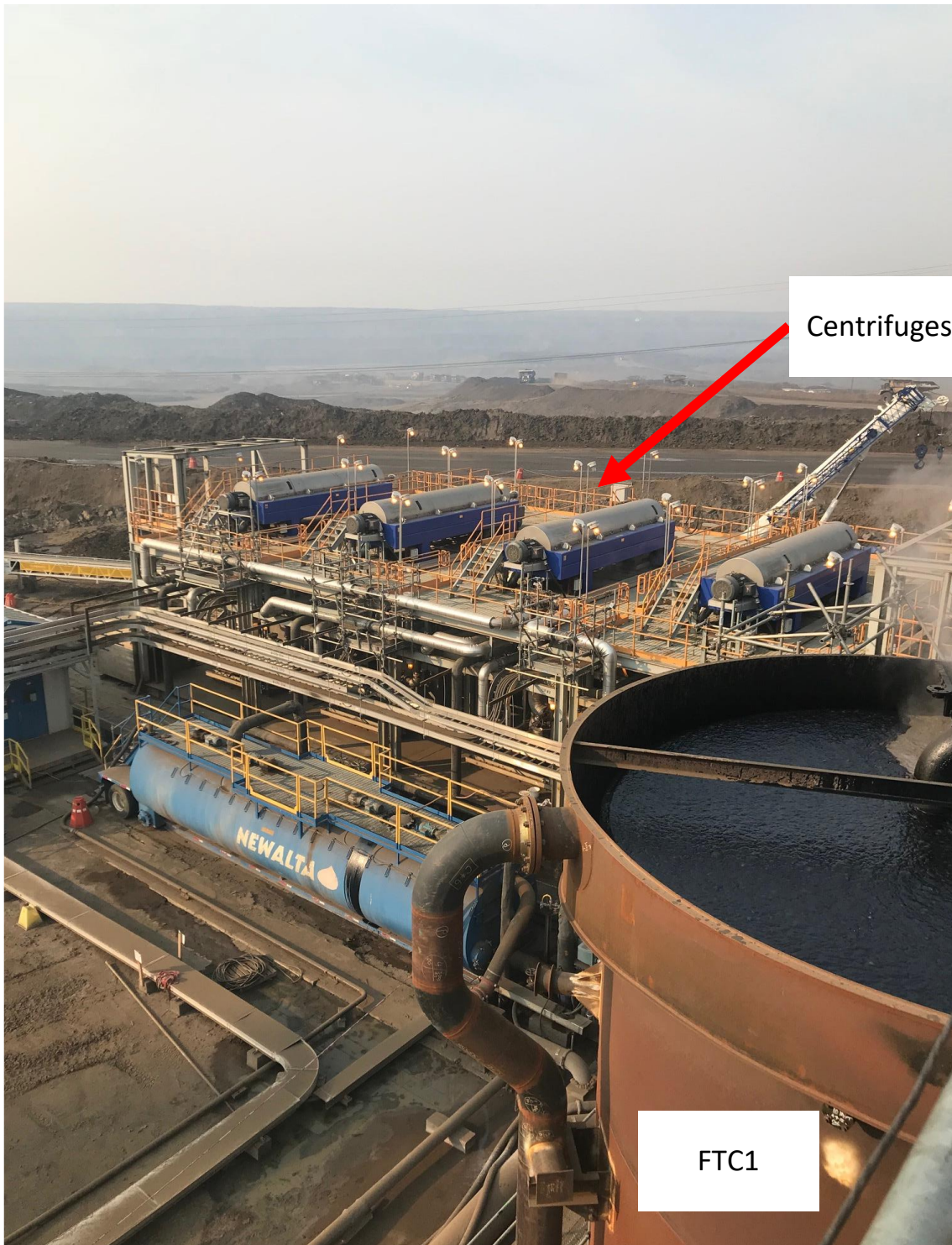
Figure D-16 Centrifuges and FTC1 during operation (Phase 1)
