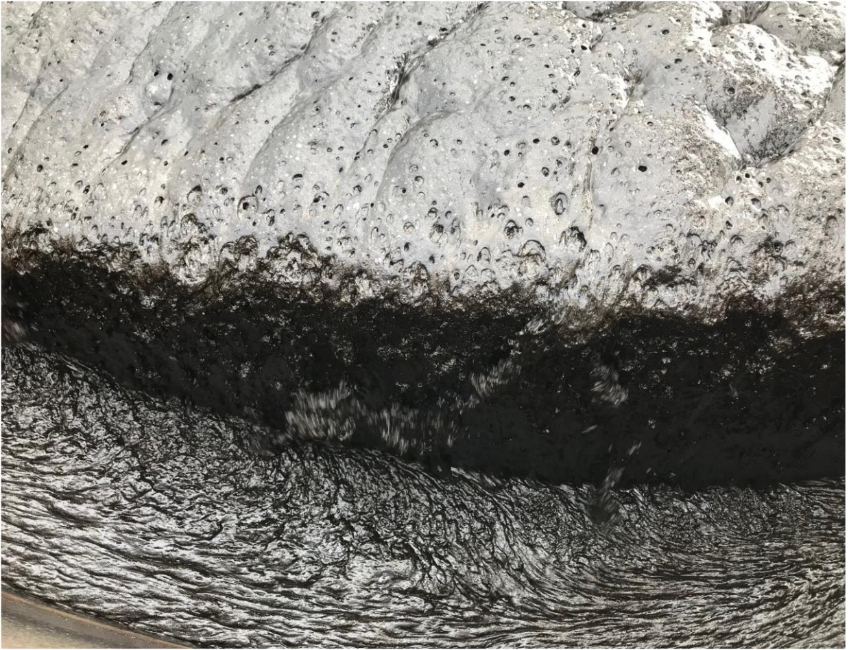
Figure D-13 Froth overflow from flash flotation cell
