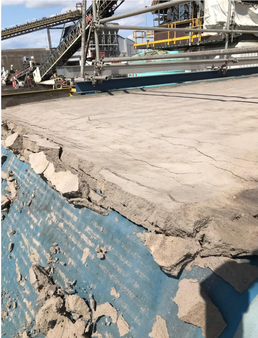
Figure D-15 Belt filter cake falling from cloth at discharge to a tailings conveyor (not shown) (Phase 3)
